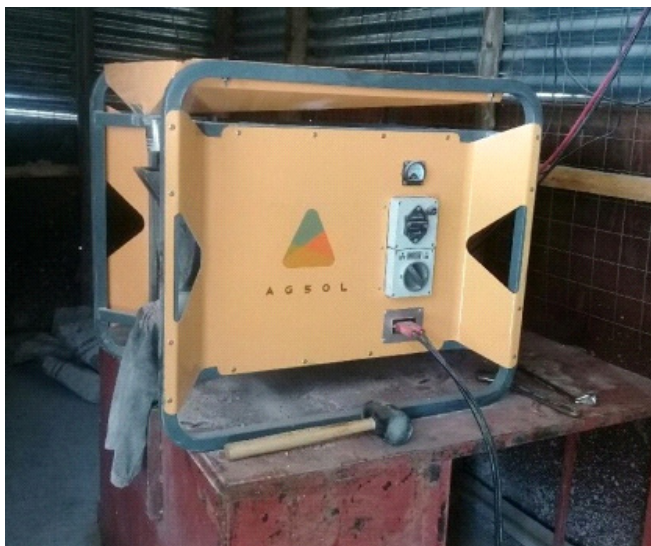
Figure 11: Solar mill in business premises.
